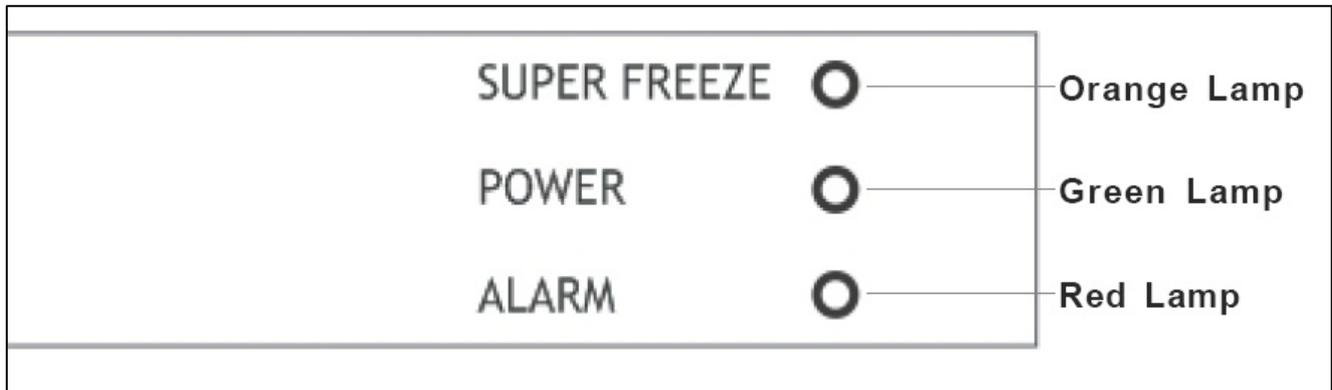
**ORANGE LAMP** : When the “Super Freezing” operation is on (thermostat dial is in SF position), the orange lamp will turn on.
